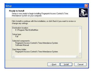
After enter into this interface, it is show that you have finish all configured to setup, if want to modify it, Click **Back** to return, Otherwise click **Install**, the installing program will copy and write corresponding information into hard disk, After finish installation, click **Finish** to complete the process.
