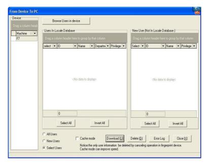
Select a fingerprint machine No. to download user's information which is on the left side list, click **View User in the Fingerprint machine**, it is able to display all user in the fingerprint machine, Select a user to be downloaded, click the "**Download**" button to download the user information and fingerprint from fingerprint machine to local database
