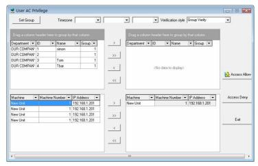
10 after users and equipment is selected, click on "allows" button, the group Time period which is used by user in the critical periods will be assigned to the selected devices. After distribution is successful, prompt will appear shown as following
