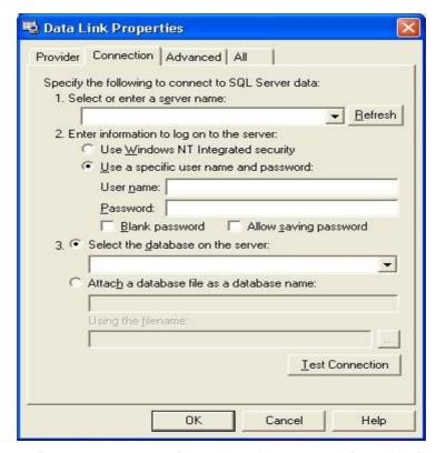
Confirm the server name for storing this database, information for logging on this serve, and the database name. After run test connection successfully Click (**OK**) button to complete settings
