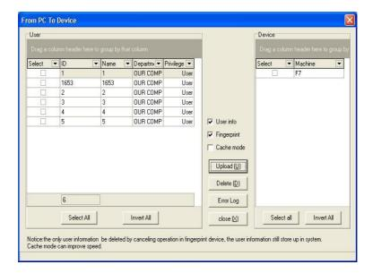
**Upload:** Base on your need, Select a staff and an uploading fingerprint machine, click **Upload**, it is able to upload user's data to the defined fingerprint machine.
