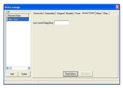
Delay time of lock control apply to determine unlock hour, the min measured unit is 20ms, in the normal condition is 100—200ms.
