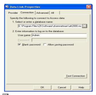
Click button, Can select the database file, the default name is att200.mdb, according to real condition to renew setup of the database connection.
