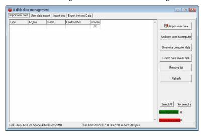
Click **Load the User Data from the USB disk** button. The system will automatically search the user data and load it into the system from the USB flash disk, if a new use is found, the system will prompt whether add the new user to system or not.
