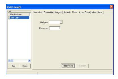
Firstly read the parameter of **Power Management**, modify the state of **Idle Setup** and minutes of **Idle Time**, then click the **Application Option** to complete set. When the idle time is 0, then the idle setup function is invalid. When the value more than 0, the machine will enter into idle state after arrives at define time.
