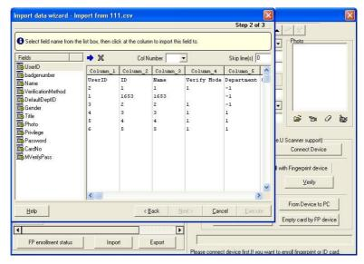
The left side list is a field list, the right side is a import file rank, there are Skip line(s) on the right-up part, that means want to skip amount of the line, if the first line to be import isn't material data, you can fill 1 here, that show to skip the first line to import data.
