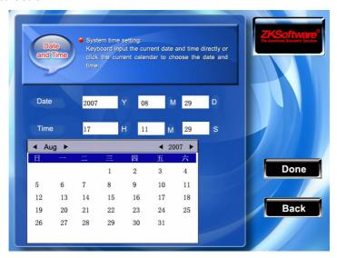
Scroll the  $\blacktriangleleft/\blacktriangleright$  key to switch option input box, Scroll $\blacktriangle/\blacktriangledown$ key to shifts the cursor input box . set up the value with the numeric keyboard input After you set up completed, please press // "OK" (F7) to save this configuration, press the ESC (F8) key to abandon operation and return to the up page
