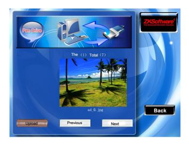
Plug the USB flash disk in the USB slot of the card machine, scroll "▲/▼" key to preview the picture in the USB flash disk then press the OK key to choose the picture you want to upload. If the prompt "upload successfully" is displayed on the equipment, the file will automatically jumps to the next picture. After completing uploading the pictures, press ESC(F8) key to exit.
