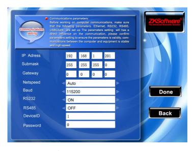
Scroll the ▲/▼、 ◀/▶key to shift the cursor on the item you need set, scroll the ◀/▶key again to shift the value which you choose. After setting up, directly press 爲 / "OK" (F7) key to save this setting and return to preceding interface, press the "ESC"(F8) key to cancel.
