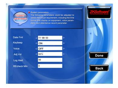
Scroll the ▲/▼ key to shifts the cursor on the item which you need set. If the item is inputting box, configure the value with the numeric keyboard input; If the item is rolls the frame, Scroll the ◄/► key to choose the value you need, after the setting finished, please directly press OK or ★/← (F7) key to save this item and return to preceding interface, press the ESC (F8) key to give up operation and return to interface.
