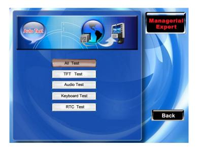
Scroll the  $\blacktriangle/\blacktriangledown$  key to select the item that needs to be tested, press the "OK" key to start the testing
