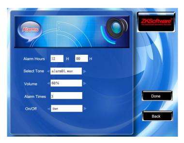
Scroll the  $\blacktriangle/\blacktriangledown$  key to shift the cursor to input box, set up the value with the numeric keyboard input. After the setting, directly press OK or the  $\rlap/\rlap/\rlap/\rlap/\rlap/$  (F7) key to save the settings and return to preceding interface, press the ESC(F8) key to give up.
