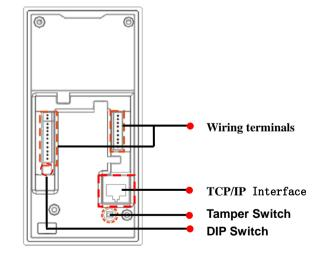
Wiring Terminal: Connects with locks and power supply through cables.
