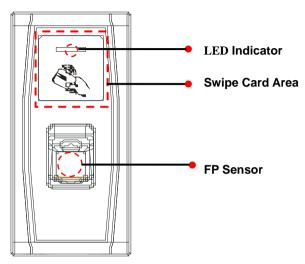
LED indicator: The LED indicator is used to display device operation results and exceptional statuses which are defined as follows:
